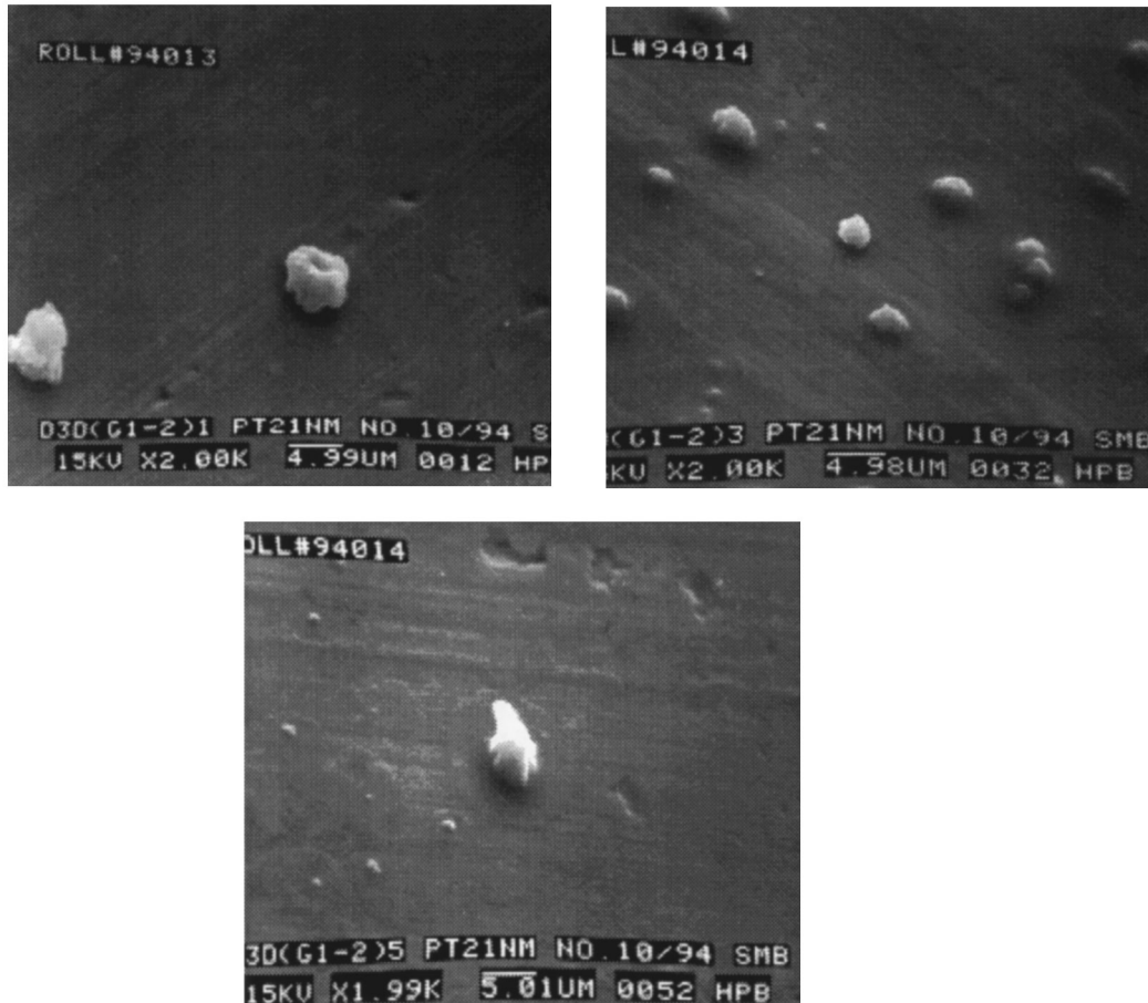
Fig. 4. Electron microscope photographs of product G. Top left, stage 1 (5.8–9.0 \mu\text{m} ); top right, stage 3 (3.3–4.7 \mu\text{m} ); and bottom, stage 5 (1.1–2.1 \mu\text{m} ). Bar = 5 \mu\text{m} .
